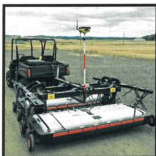
Above: the STREAM C demonstrated by IDS-NA targets underground utilities for base mapping. Credit: IDS.
