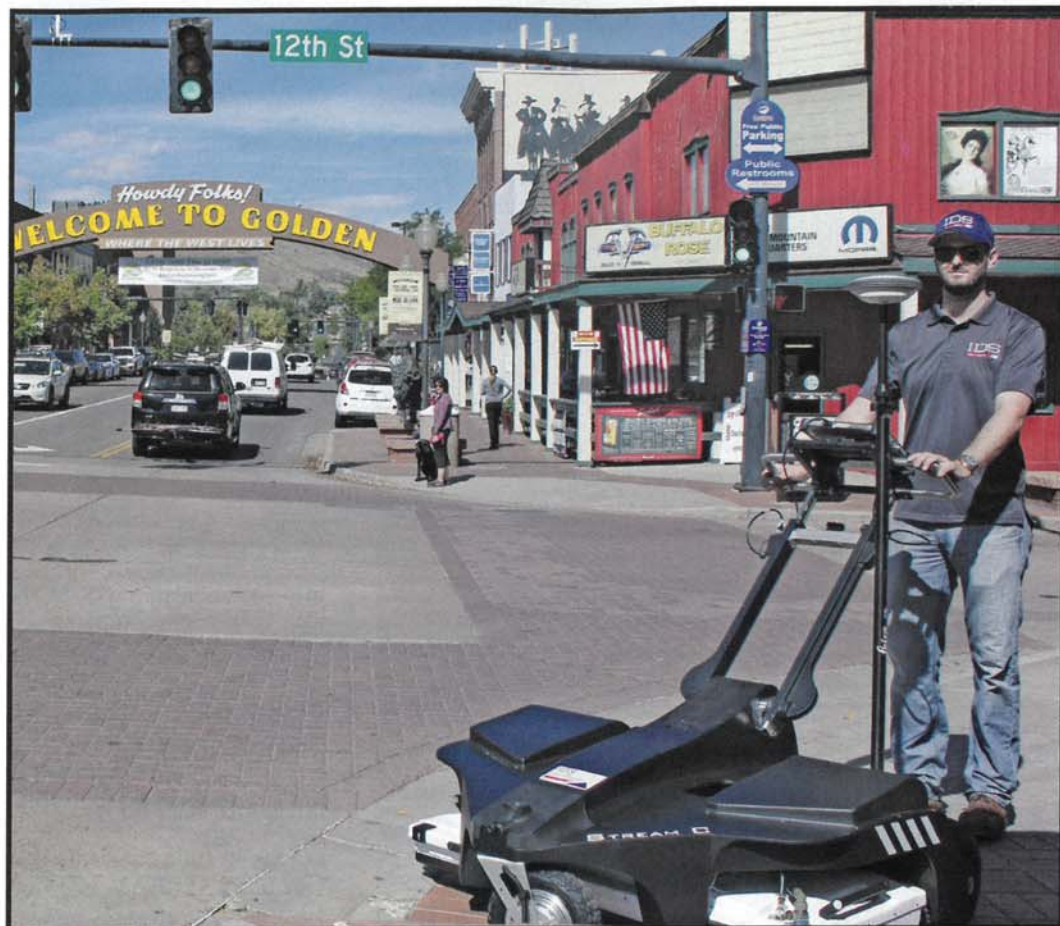
Above: the STREAM C demonstrated by IDS-NA targets underground utilities for base mapping. Credit: IDS.
